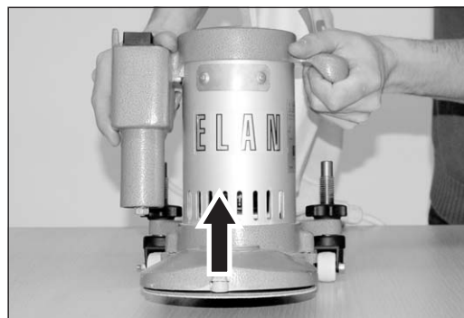
Fig. 10 Always tip the machine backwards slightly before switching on or switching off the machine.
