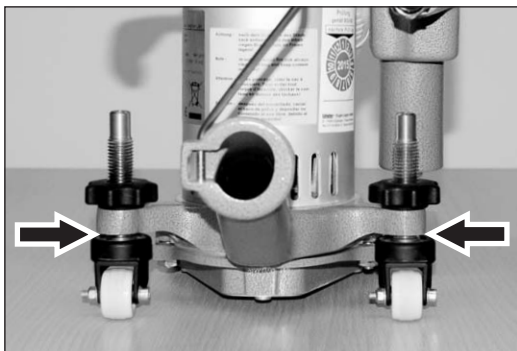
Fig. 57 Flat machine setting for fine sanding tasks.
