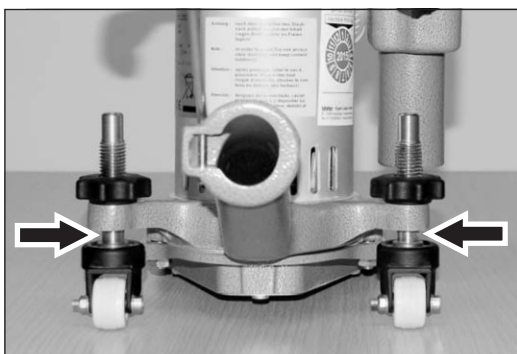
Fig. 59 Steep machine setting for rough sanding tasks.
